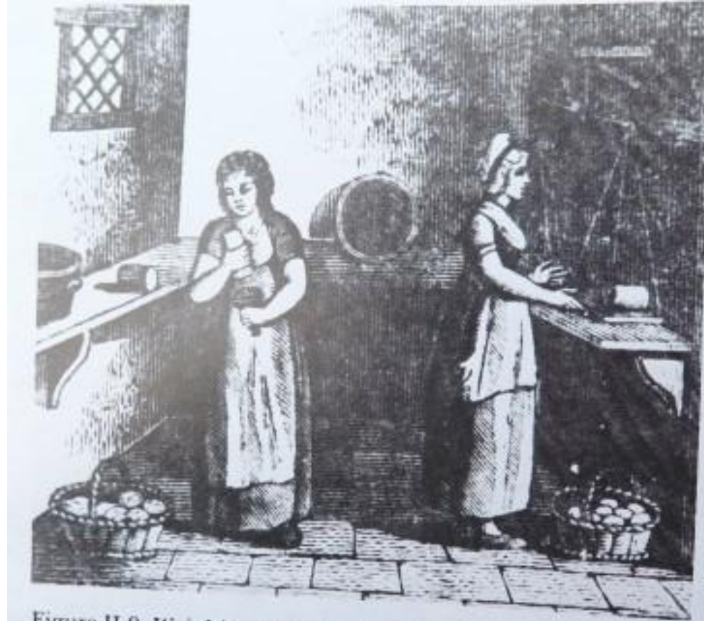
Figure II-9. Weighing and printing. One woman has a roll of butter on a scale. The other woman holds a wooden print in her left hand and removes the printed butter with her right hand; the printed rolls are in her basket.
